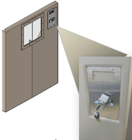
1. The door handle will pop out when unlocked. If it does not pop, try a second key. If it still does not pop, reach inside the door and press the latch "tab" with a screwdriver. The door handle will pop and the latch should operate.
