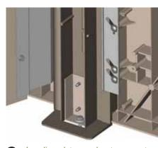
**C** Leveling plates anchor to concrete pad (or C-strut) with stainless steel expansion anchor bolts to allow 3" of vertical adjustment.
