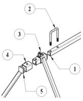
12465 - Support Bar 2 12464 - U-Bolt 12457 - Inner Leq 12456 - Outer Leg 12466 - End Cap
