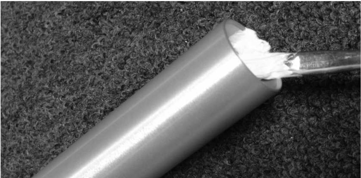
13. Install piston seal into cylinder.
