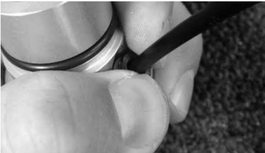
6. Using a screwdriver, push the pressure gauge out of the gauge housing
