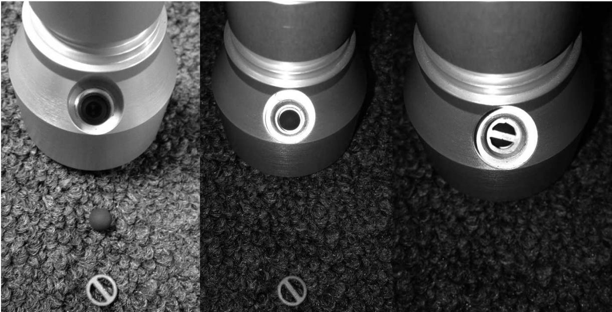
17. Apply thread sealing tape to fitting and reinstall with 1/8" hex key.
