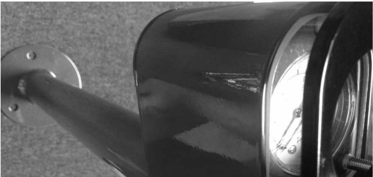
26. Install and tighten the nuts to the top cap. To make this easy, load a socket as shown so that the threads are easily started.
