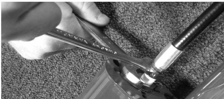
29. Test the pump by inflating a bike tire. Leave the pump connected to the pressurized bike tire and listen for leaks.
