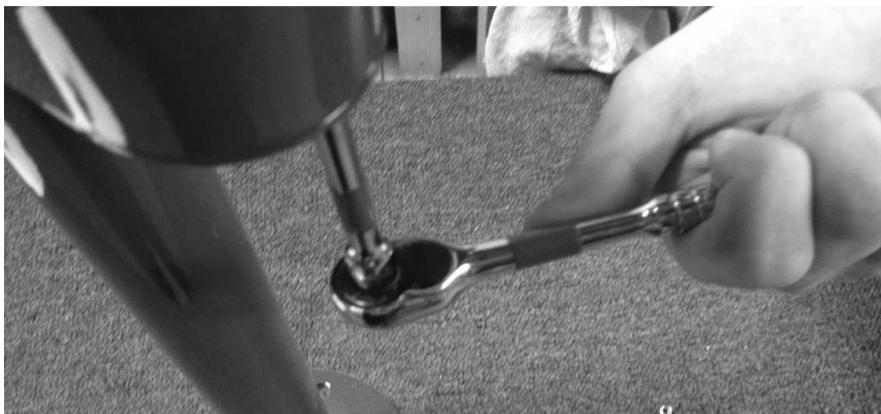
4. When all three nuts have been removed, pull the top cap off the pump. You can now lift the pump rod, bushing, and cylinder out of the pump. There is a tubing attached to the bottom of the pump. Be careful not to kink this line while removing the internal components.
