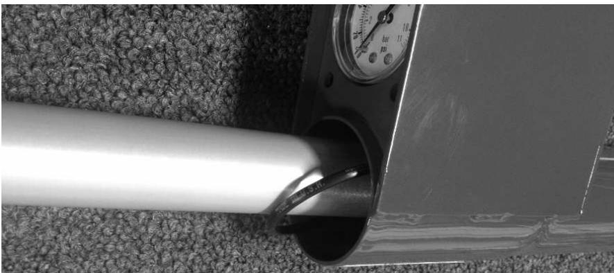
23. You will lower the assembly down. To keep the components from separating while lowering it into the pump housing, you will grab the piston rod, bushing, and cylinder while lowering as shown.
