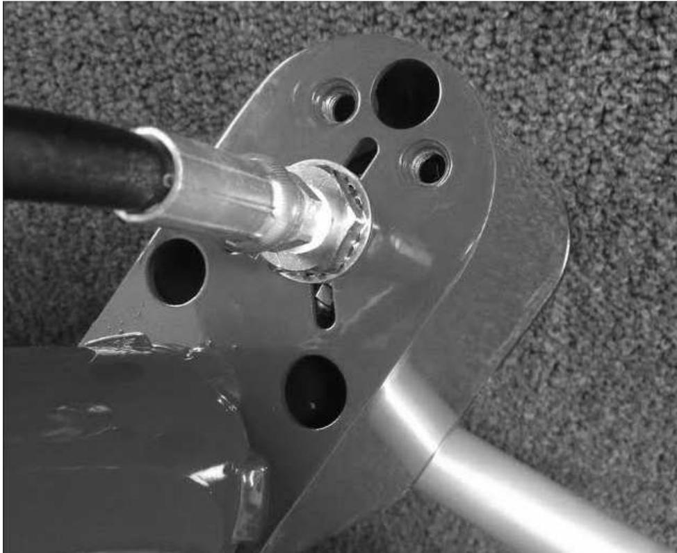
3. Using a 1/4" drive ratchet with a 6" long extension and a 10mm socket, remove the three top cap nuts.
