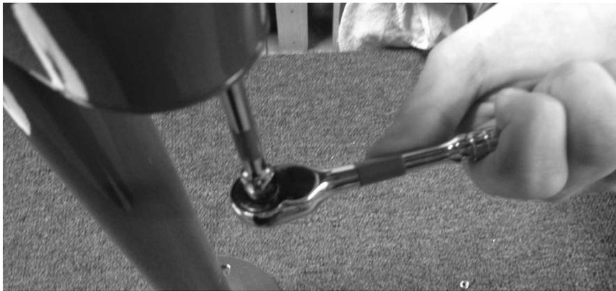
28. If you need to replace the hose, use a large adjustable wrench and a 9/16" or 14mm wrench to remove the hose. **NOTE: Do not attempt to remove hose without an adjustable wrench to react the torque or the gauge will spin.**
