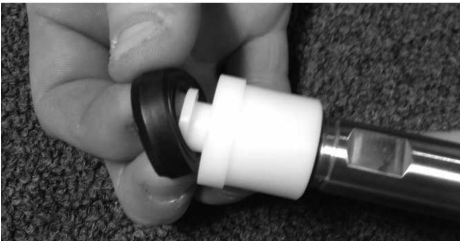
11. Lubricate new piston seal with provided grease.
