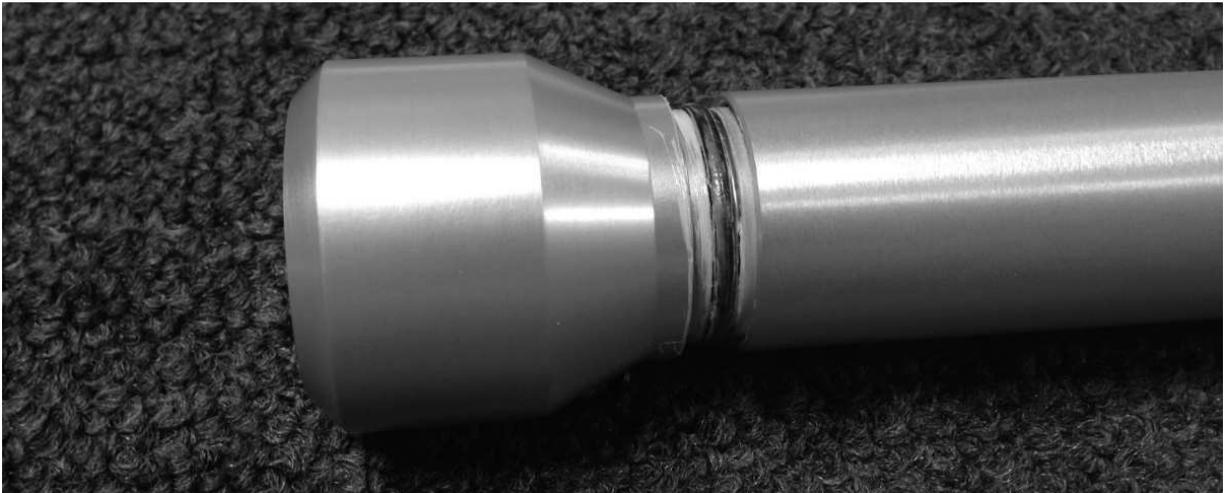
15. Remove fitting using 1/8" hex key.
