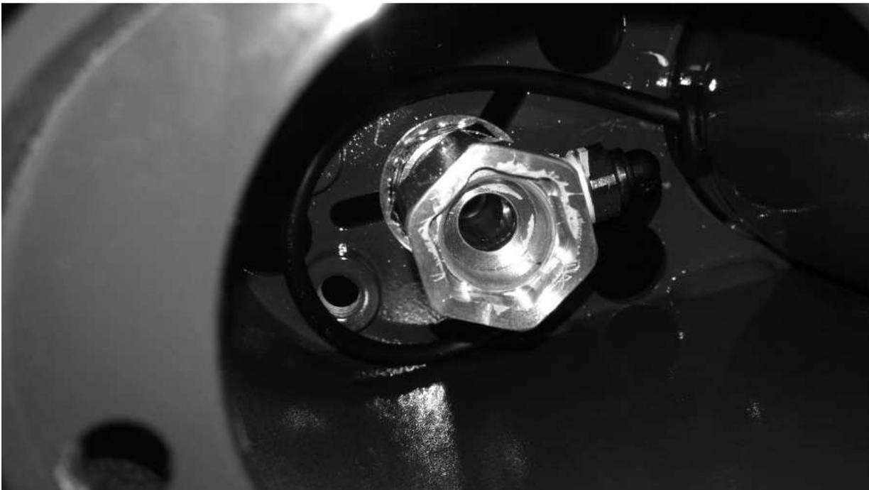
21. Connect the tubing to the footvalve.
