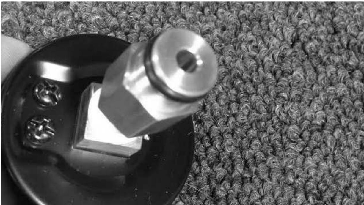
8. You can now remove the piston and rod from the cylinder.
