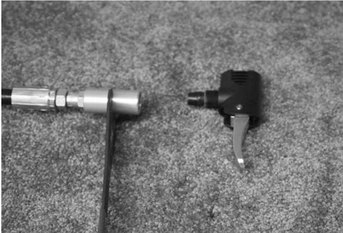
4. Make sure replacement Air Chuck has a rubber stopper on the plastic nipple. Rubber tube is attached in photo A and not in photo B.
