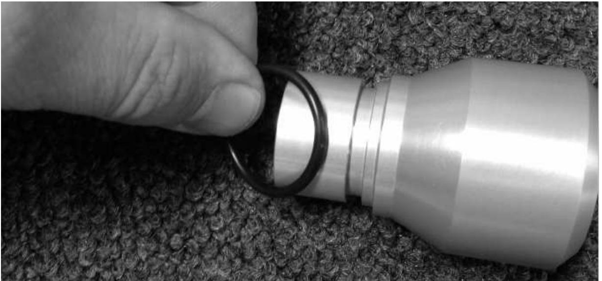
19. Grease and reinstall fitting
