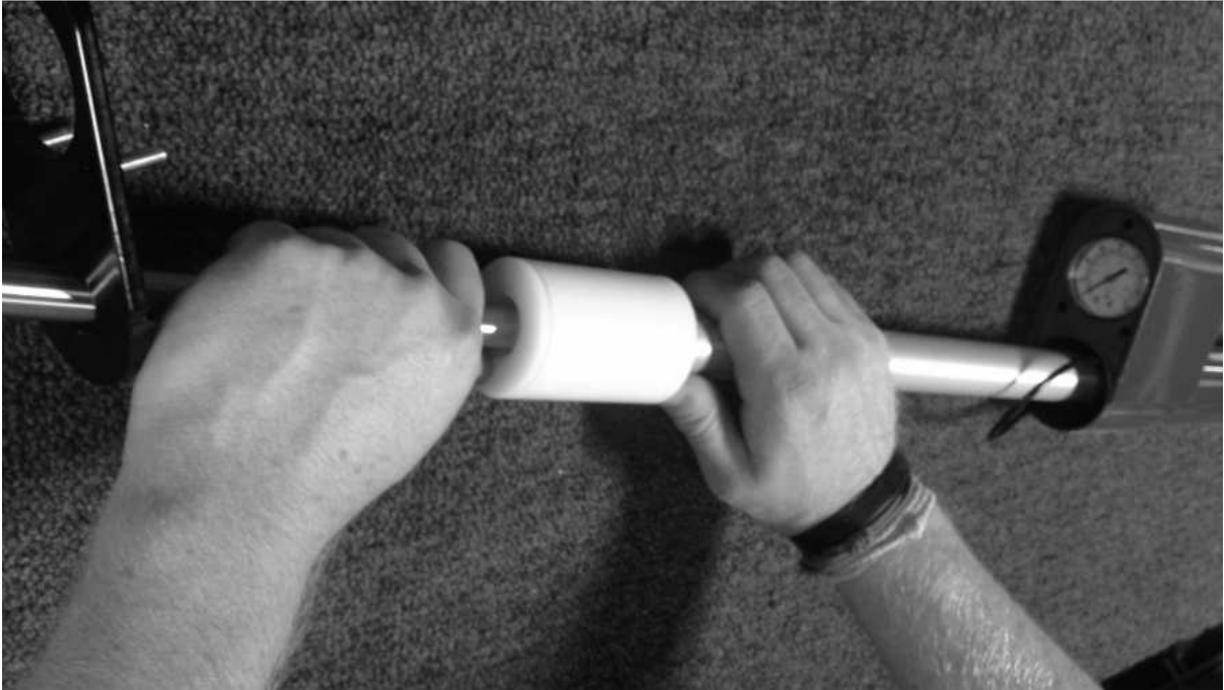
5. In order to disconnect the air line from the foot valve at the bottom of the pump, you must depress the tabs of the fitting and then pull on the hose.
