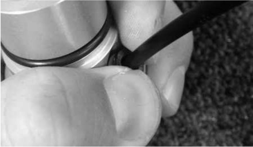
22. Begin installing the pump's internal components into the housing as shown. **NOTE: Slowly install assembly to avoid kinking the tubing.**
