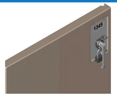
**#10720 ProPark Swing Handle**. Padlockable handle with spring return includes bracket to secure user-supplied padlock or bicyclist U-Lock (cyclists or owner to provide lock) to replace T-Handle. Zinc coated/heavy duty construction handle or stainless steel handle upon request. Intended for open-access bicycle lockers.
